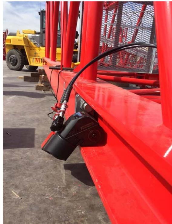
Figure 3: Test with the hydraulic torque multiplier AT from alkitronic.
