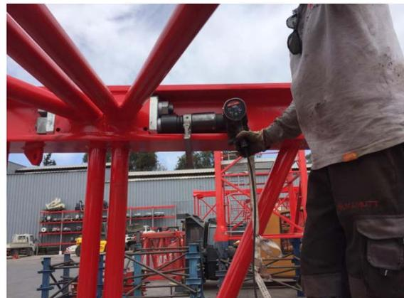
Figure 1: The angled electric torque multiplier ECWip100 from alkitronic on the crane bolting connection.
