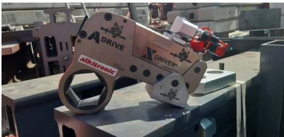
Figure 4: The alkitronic X Driver with its flat design is ideal for working in tight spaces.
